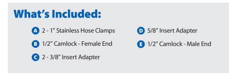
One Camlock Connector Kit will be needed for each airline connection between the manifold flex tubes and underground airline runs.
