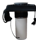
Down Tube (float not included) fit F750DP, & F1000DP 23 1/2" shroud extension, which attaches to aerator unit to pull water up from deeper depths.
