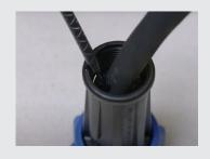
**12** SLIDE the end nut up to the quick disconnect body tighten completely. If potting compound does not pool at the top of the end nut, fill the remainder with potting compound as needed.
