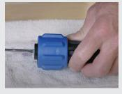
**10 PURGE** the first 2-3 mls of the 50ml tube of potting compound into a bag or cup to ensure a proper mixture.
