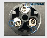
SLIDE the quick disconnect body up to the receptacle, then turn the disconnect body counterclockwise and hold the receptacle in place with a flat screwdriver in the center slot. DO NOT spin the receptacle with the screwdriver; this will cause the wires to twist and pull out of the terminals. The receptacle should be flush with the end of the disconnect when secured.
