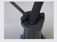
1 3 ALLOW potted quick disconnect to cure for a minumum of 45-60 minutes, making sure to keep the disconnect and cord in the upright position.
