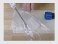
**1 1** FILL the disconnect body while keeping it in the upright position. Fill until the last 2-3 threads are still visible inside the end of the disconnect.
